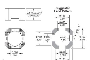
\*Dimensions are of the case not including termination. For maximum overall dimensions including the termination, add 0.010 in / 0,254 mm.
