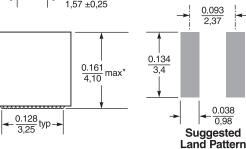
\* Height dimension shown is for the mounted part after reflow. Dimension before mounting can be an additional 0.005 inch / 0,13 mm.
