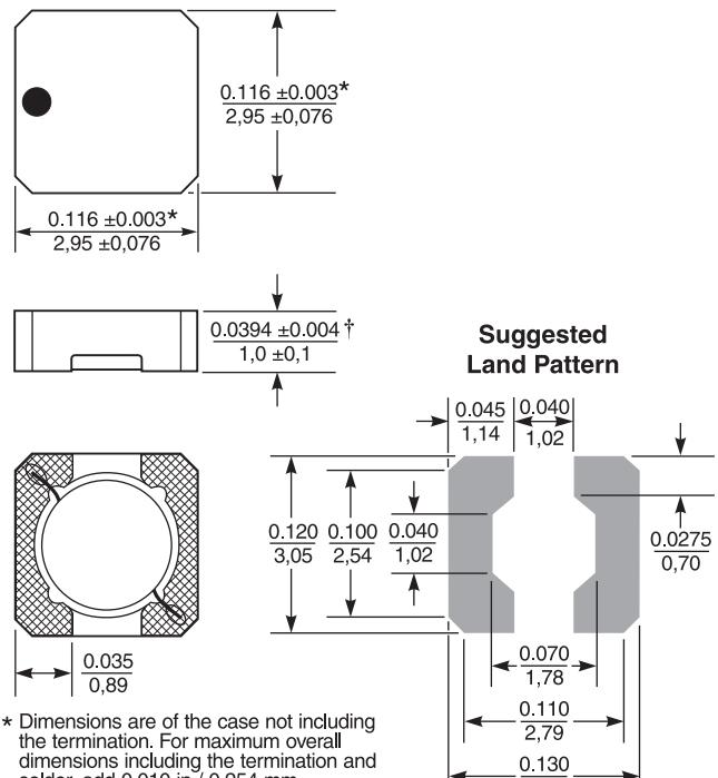
\* Dimensions are of the case not including the termination. For maximum overall dimensions including the termination and solder, add 0.010 in / 0.254 mm.
