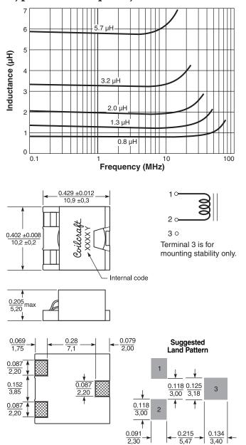
Dimensions are in  $\frac{\text{inches}}{\text{mm}}$
