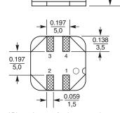
\*Dimensions are for the mounted part. Dimensions before mounting can be an additional 0.006 inch (0,152 mm).
