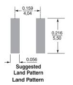
Dimensions are in  $\frac{\text{inches}}{\text{mm}}$
