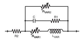
The value of the frequency-dependent variable resistor R<sub>VAB1</sub> is calculated from:
